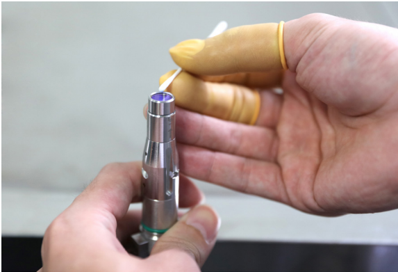
7-3 Cleaning protective lens with swabs
